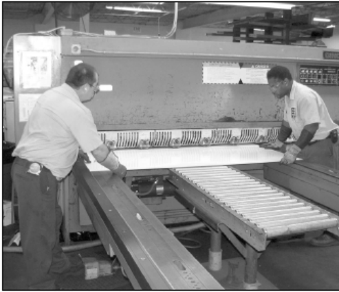
Aluminum Line Products employees Bob Beauregard and Mike Jones cut a sheet of aluminum on a CNC shear. (West Life photo by Kevin Kelley)
